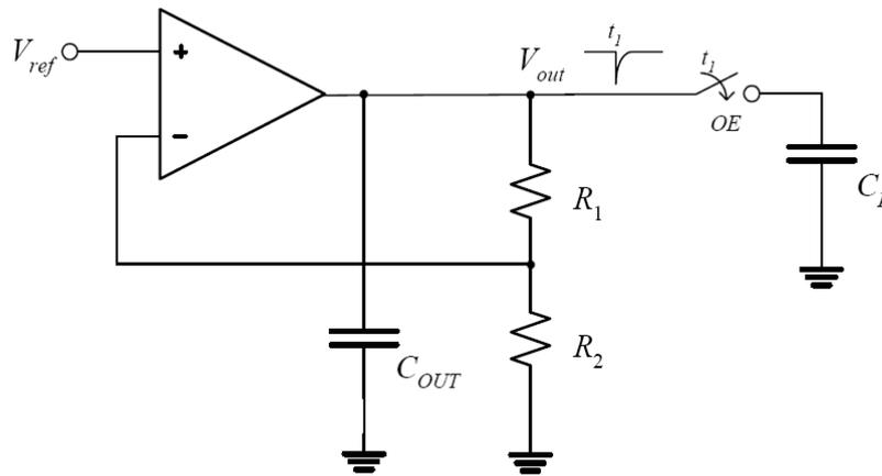
Fig. 2: Typical voltage regulator scheme.
