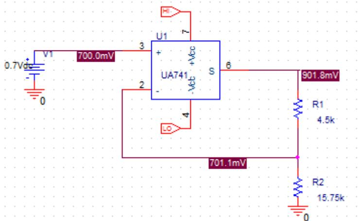
Fig. 3: Voltage regulator scheme using Pspice.
