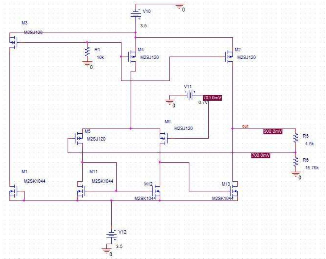
Fig. 8: Voltage regulator scheme using NMOS transistors using Pspice.
