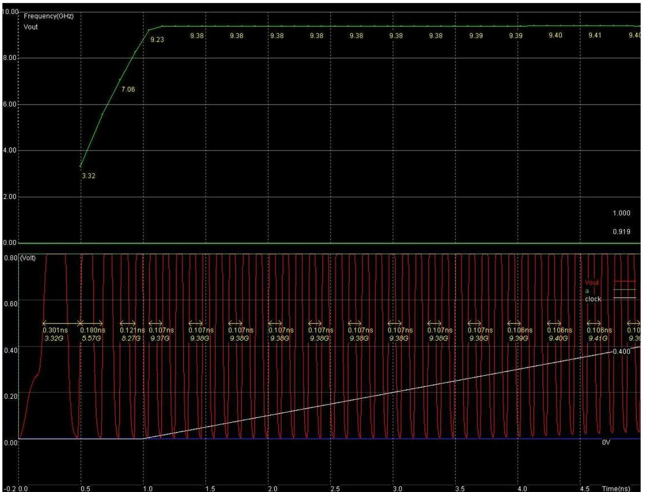
The simulation shows the response in frequency obtained and we can see that the oscillator has a bandwidth included between 3,32GHz and 9,25GHz. It's linear to 9,25GHz and after the oscillator is saturated, so it's useless to increase the Vdd voltage of the regulator.
