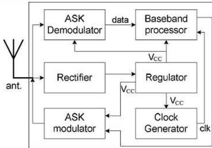
Fig. 1: Passive UHF RFID tag diagram.
