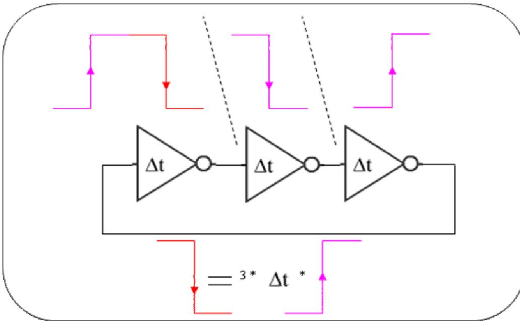
We use inverters logic gates to toggle the signal and as a gate as a delay, we can make a constant output frequency. So the output frequency is then a function of the delay in each of logic gates. Of course we must use an odd number of gates to make an oscillation.
