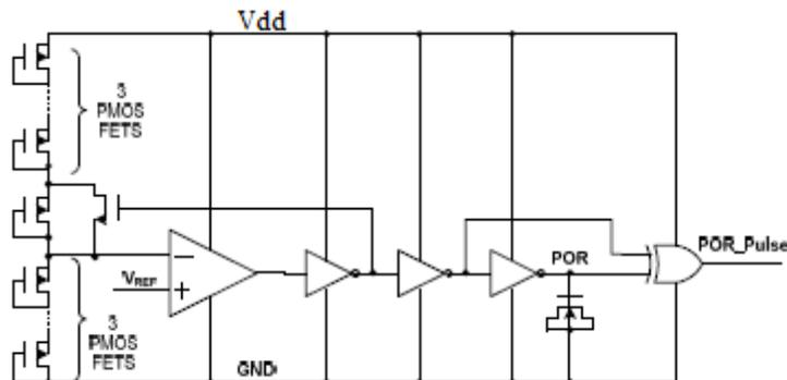
Fig. 11: Power-on-Reset circuit scheme.
