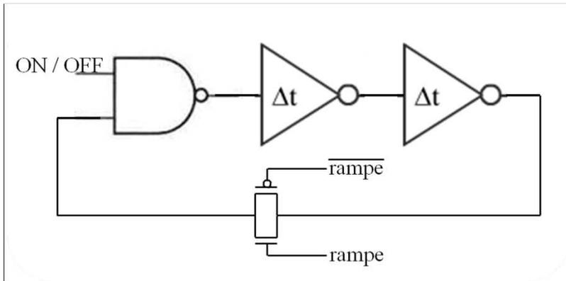
We find again our logic gates which make a delay in the signal. An inverter was replaced by a NAND to activate or not the oscillator. And the particularity is the ramp.
