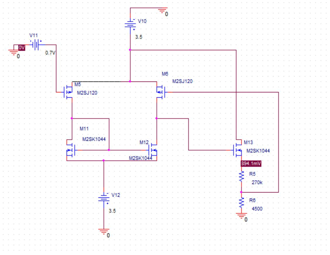
Fig. 4: Voltage regulator scheme using NMOS transistors using Pspice.
