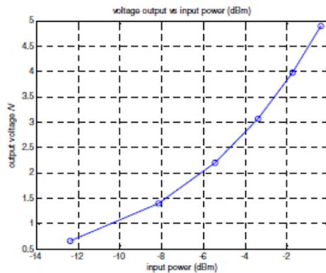
Fig. 7: Output voltage vs. Input power.
