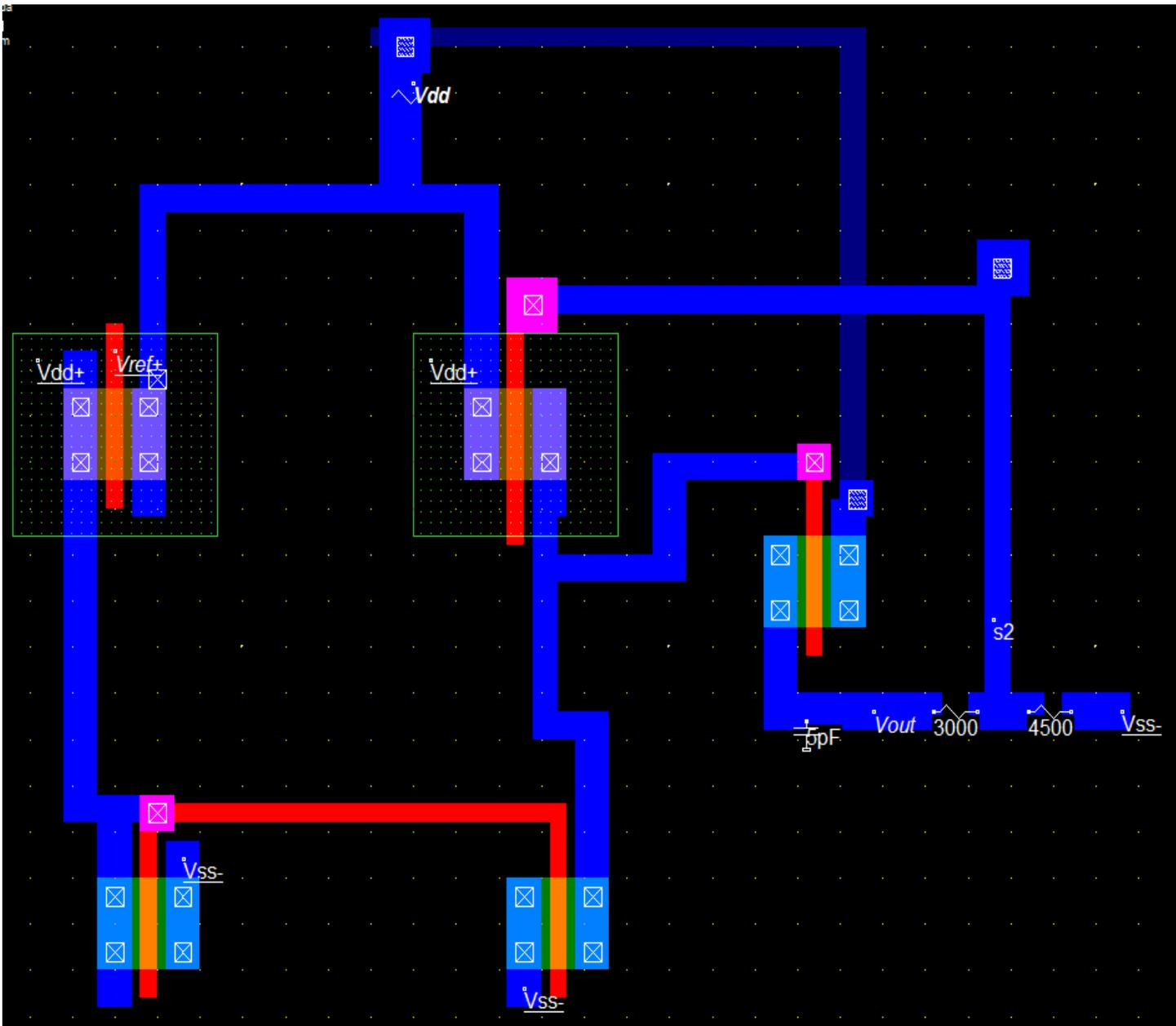
Fig. 5: Simple Voltage Regulator design using Microwind.
