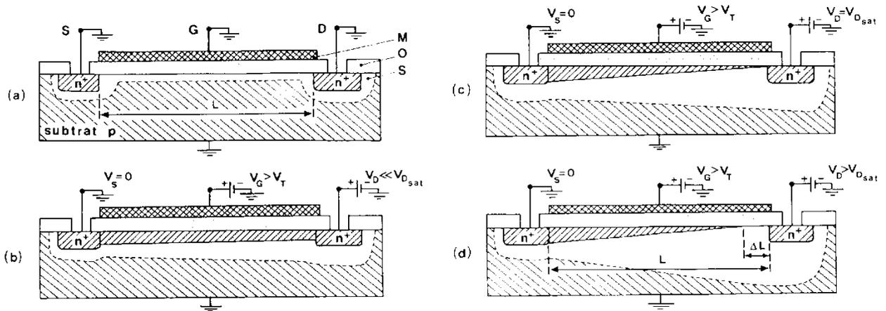
*Principle of the creation of the channel of a transistor MOSFET.*
