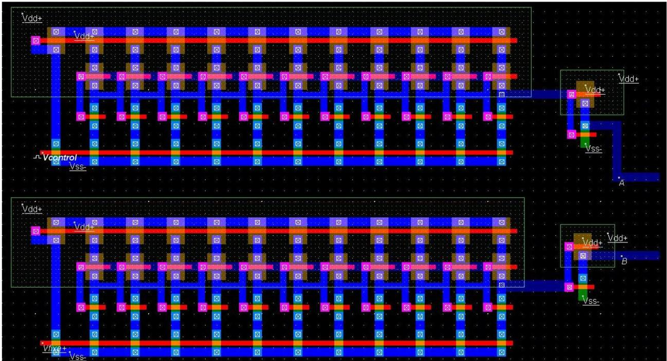
Two VCO's were added in order to create two different waves for comparison in the output. The first one was controlled with a variable tension  $V_{control}$  and the second one with a DC tension  $V_{fixe}$ . With this setup, the simulation has given the following results.
