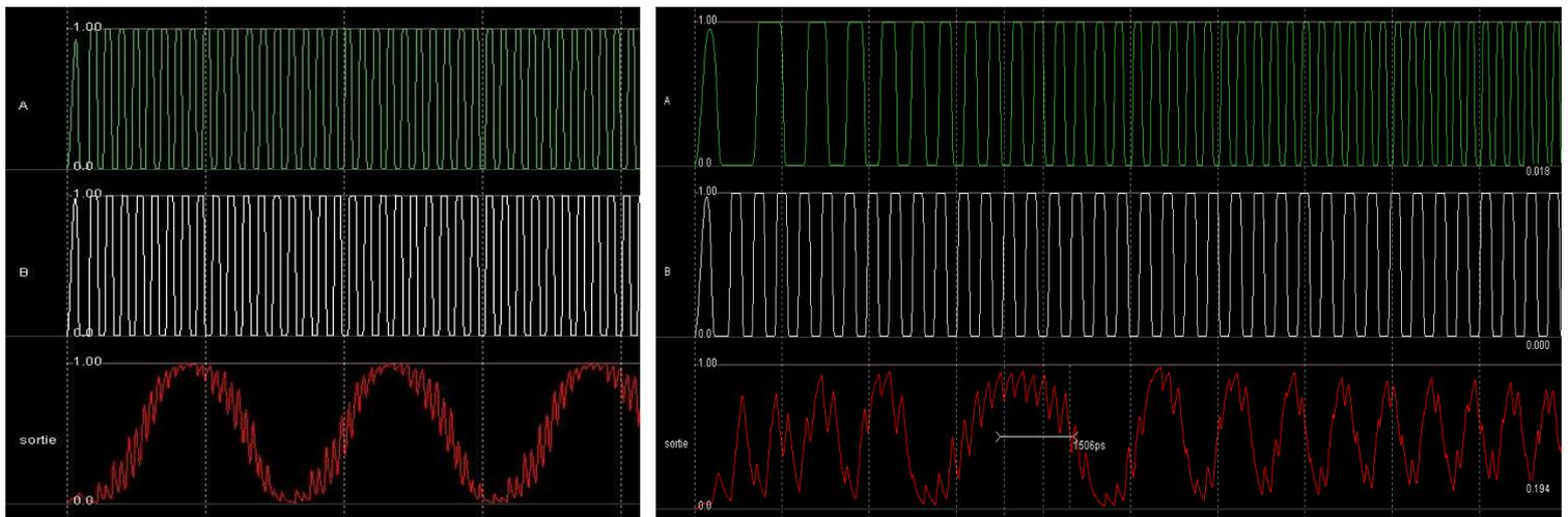
Due to the choice of the capacitor, we did not obtain a perfect signal, but we can confirm its periodic aspect. Furthermore, its frequency goes up when the two in input move away. It is also important to notice that the final output frequency is equal to the difference between the two from the VCOs.
