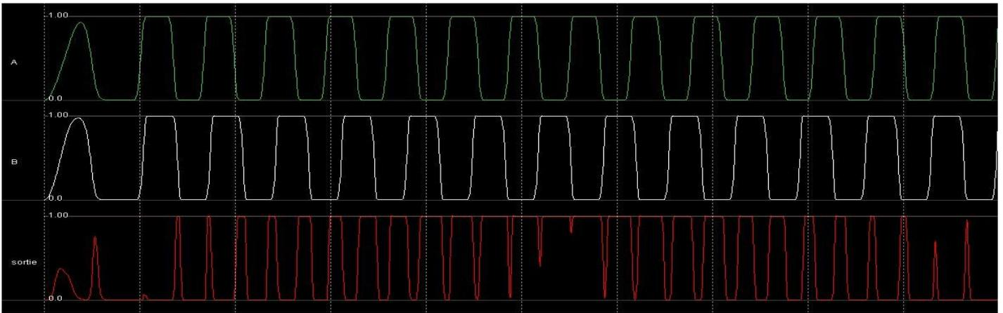
We can see a variation of a duty cycle, which increases then decreases. This structure of the signal is repeated, so we can hope that with a capacitor, there will be a periodic signal in output.
