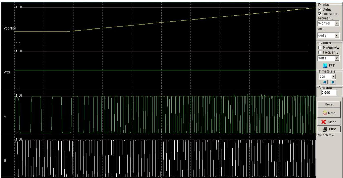
As expected the output of the first VCO rises its frequency as  $V_{control}$  rises, and on the second VCO the frequency stays the same, creating a clock pulse.
