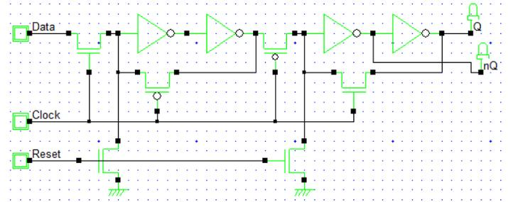
Fig. 4. Dreg configuration using inverters
