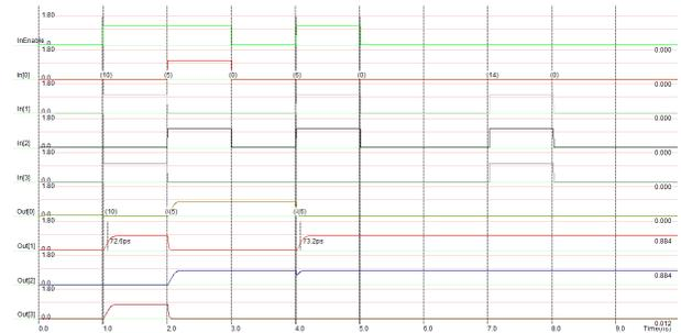
Fig. 13. Input PAD simulation. The external inputs are 10, 5 and 6 for A, B and RF input respectively and as chip inputs we have the same values. This response validates the input path.
