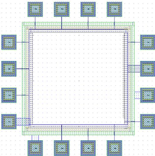
Fig. 8. Chip General Structure. For practical purposes it is presented the chip without the connection to other modules. Three ring pads are present: one for  $V_{SS}$ ,  $V_{DD}$  and  $V_{DD-High}$
