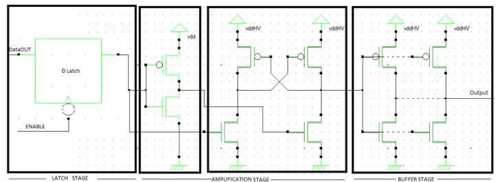
Fig. 10. Output path schematic
