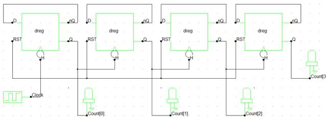
Fig. 3. Counter Schematic
