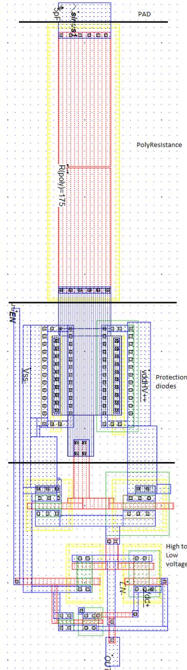
Fig. 9. Input Pad Layout. Three stages are present and a 5 pF capacitor simulates an input pad interaction
