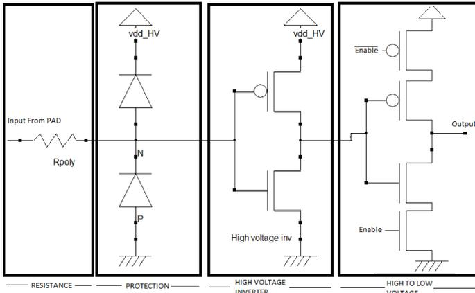
Fig. 7. Input path schematic
