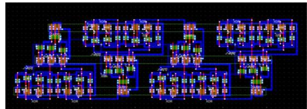
Figure 3: Layout of the 4bit adder
