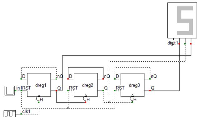
Figure 8: Schematic of the 8 bit program counter
