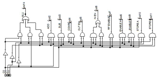
Figure 12: Schematic of the Instructions Decoder
