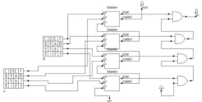
Figure 2: Schematic of the 4 bit adder
