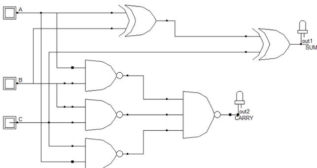
Figure 1: Schematic of a Full Adder
