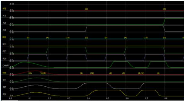
Figure 4: Simulation of the 4bit adder
