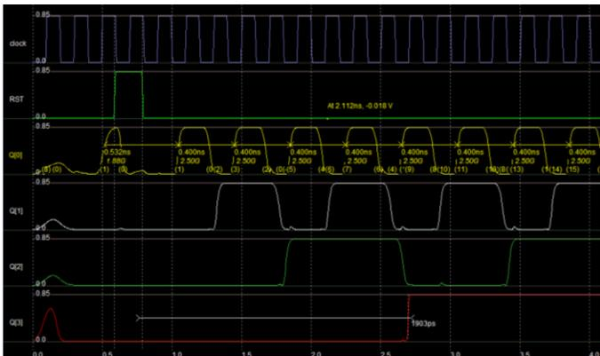
Figure 6: Simulation of the 16 bit counter
