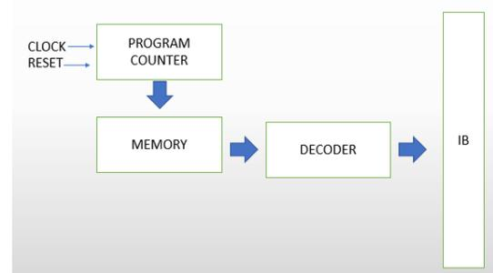
Figure 7: Flow Diagram of the Program Counter and Decoder inside the chip
