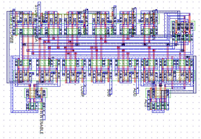
Figure 13: Layout of the Instructions Decoder
